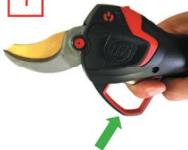
**After connecting and switching on your pruning shears, make sure the blade is closed, then press and hold the trigger, the bar graph will turn off and the ON/OFF status LED will turn red.**
